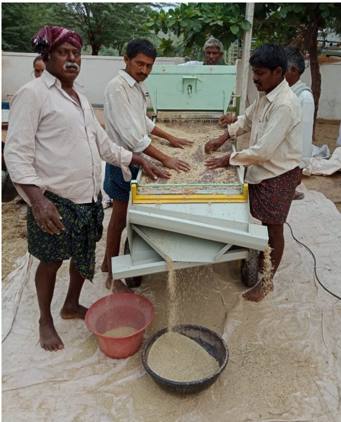
Farmers use grading machine to clean their harvest of brown top millet. Agro-waste falls off to the side from the upper deck; small grain collects in the red tub and the good grain remains in the middle deck and collects in the black tub. More info — Millet Machines and Tools Mr. Dinesh @ 94408 70875 | milletmachinesandtools@gmail.com
