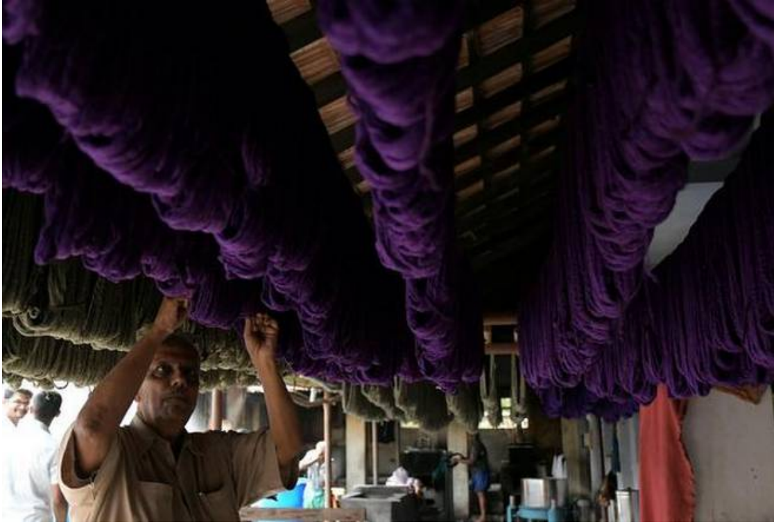
Dyed yarn is hung for drying. | Photo Credit: G. KARTHIKEYAN
